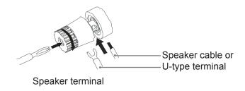
Make sure that no wires are not insulated can bypass the speaker outputs. Make sure that the speaker terminals are tight enough to ensure a good electrical connection. If the terminal screws are not tight enough, the sound quality may be affected.
