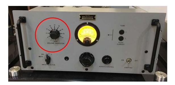
The top left knob controls the INPUT gain level all the way to infinite level. Before turning on your system, you should turn this knob all the way down to minimum then adjust from there. Do NOT leave the knob at infinite level when you turn off the system. You may accidentally damage your speakers when you turn on system next time!
