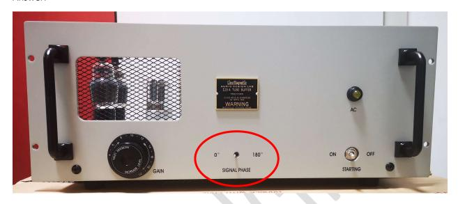
The 0 to 180 degree signal phase toggle (middle of faceplate): Nearly half of the world's recordings were recorded phase inverted. This toggle will allow users to reverse the recording phase to possibly hear better sound imaging and details. In your AS-123 Tube Buffer manual, there is a table (also copied here) showing the recording phases by different labels. Please refer to it to experiment and enjoy your music collection with newly found pleasure.
