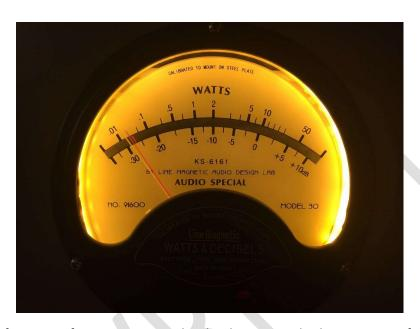
The front meter of AS-125 is for output current level. When meter display is set at 4, if the meter reading is consistently higher than 10, the playback is usually in distortion range already. In such a case, the output volume is too high and needs to turn down a bit. The front meter is a great visual addition the amp's appearance, however, for the ultimate sonic experience, factory suggest do NOT turn on meter display at all during critical listening.
