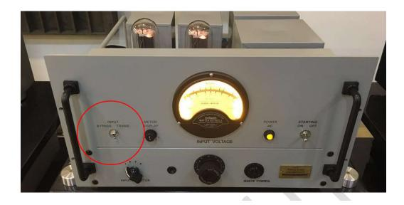
The output gain control (middle black knob) on AS-125 is wired to transformers so it cannot be bypass-wired like a typical volume potentiometer. It is suggested in bypass mode, users should set it between 12 o'clock and 4 o'clock position. A more efficient speaker will need it to be set at closer to 12 o'clock. A less efficient speaker will need to to be set at closer to 4 o'clock. In extreme situation of very difficult to drive speakers, it can be set to 5 o'clock but this not common.
