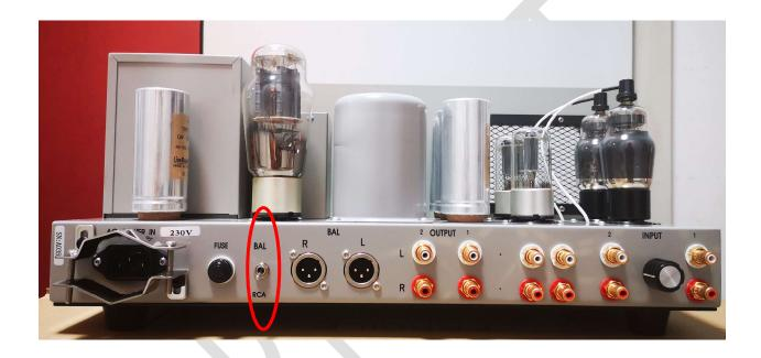
AS-123 has two types, total three sets of outputs – (2) sets of RCA and (1) set of XLR. A BAL (balanced) / RCA toggle controls which type of output is actively connected.
