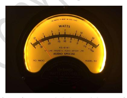
The front meter of AS-125 is for output current level. When meter display is set at 4, if the meter reading is consistently higher than 10, the playback is usually in distortion range already. In such a case, the output volume is too high and needs to turn down a bit. The front meter is a great visual addition
